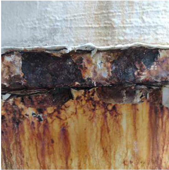
Coating Failure at a flange on the Riser Pipe
