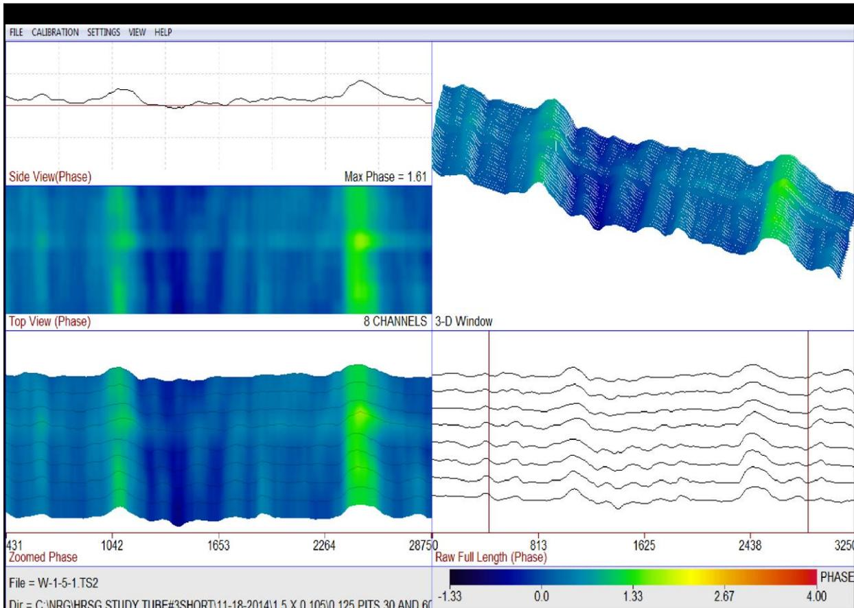
*LFT waveform above is from the study tube. The response of the 1/8" pits is circled with the 30% being on the left and the 60% on the right.*
