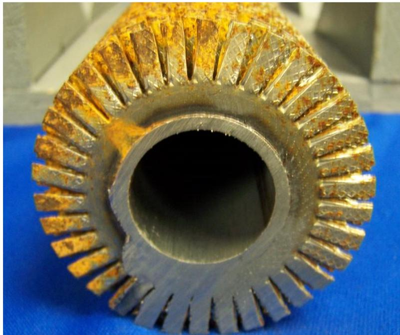
The picture shows the fins attached to the outside diameter.
