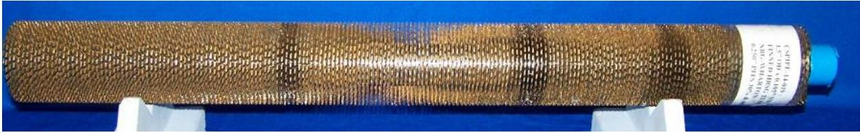
The picture above shows the study tube which has 1/4" diameter pits machined on the inside surface. The first pit is 30% deep and the second pit is 60% deep.
