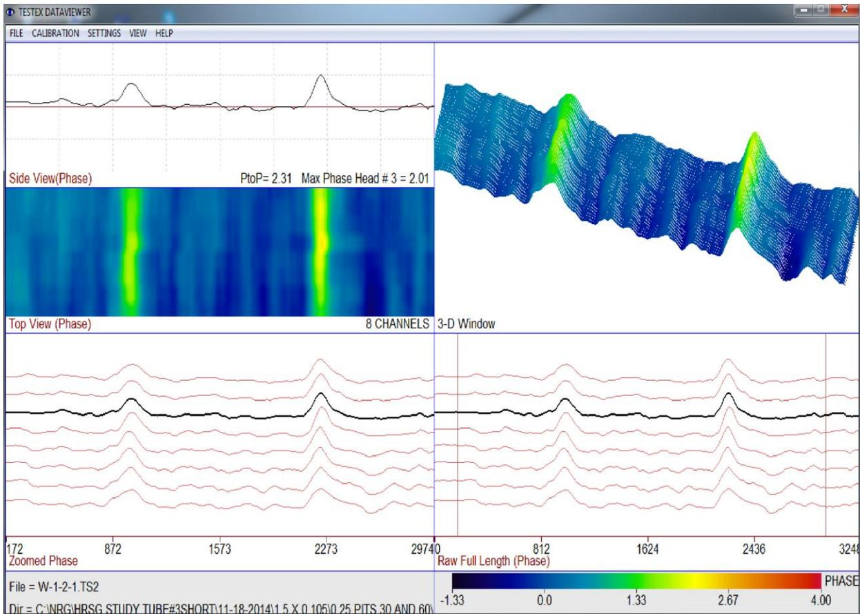
The LFET waveform above is from the study tube. The response of the 1/4" pits is circled with the 30% being on the left and the 60% on the right.
