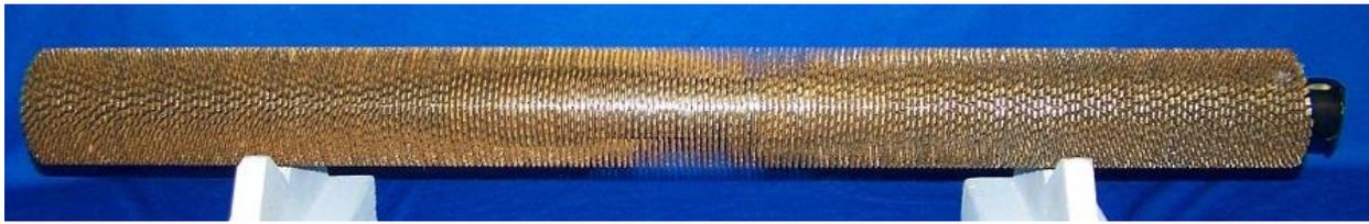
The picture above shows the study tube which has 1/8" diameter pits machined on the inside surface. The first pit is 30% deep and the second pit is 60% deep.
