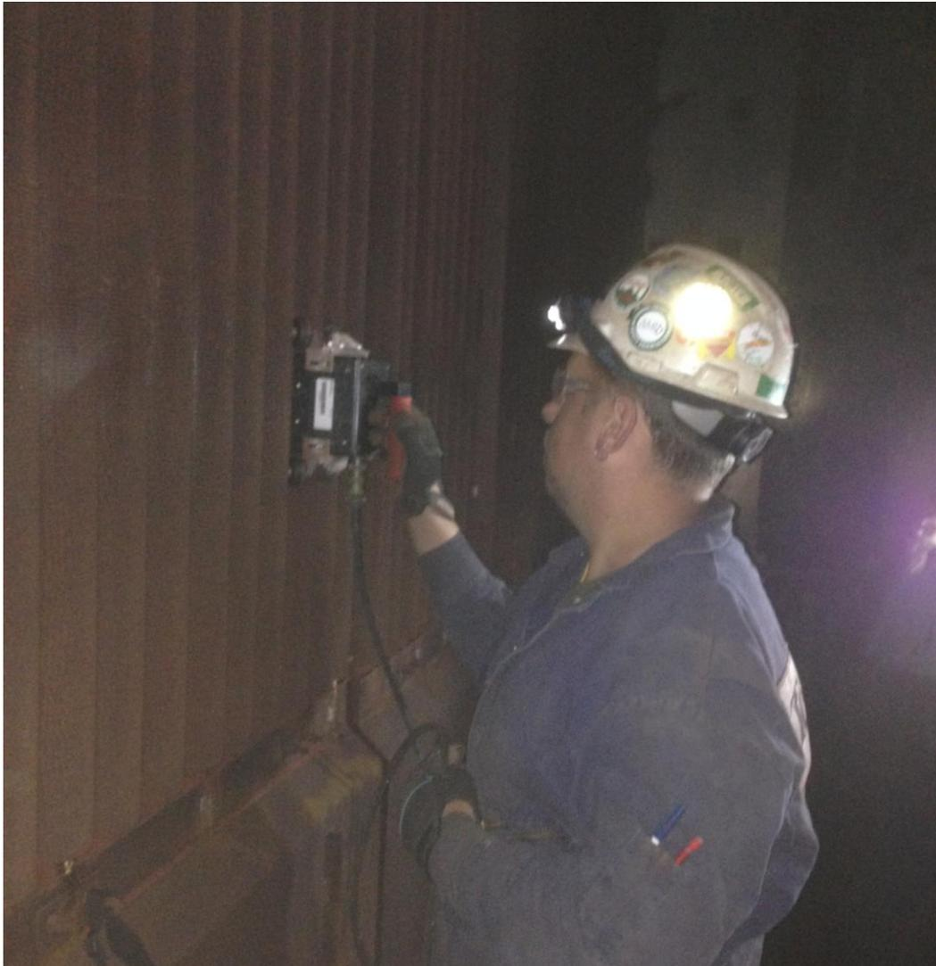
*The picture above shows a finned HRSG tube being scanned with an LFET Scanner to measure the wall thickness.*
