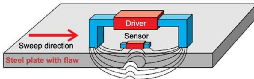
With flaw, sensor sees distorted magnetic field near the flaw as probe sweeps across the plate.
